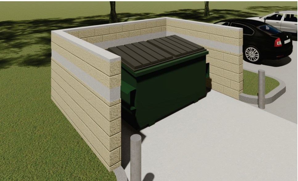
Concrete block screen around dumpsters to match building block
