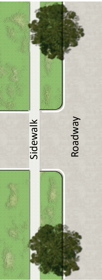
Exhibit C06-16. Sidewalk/Driveway Interface Treatment
