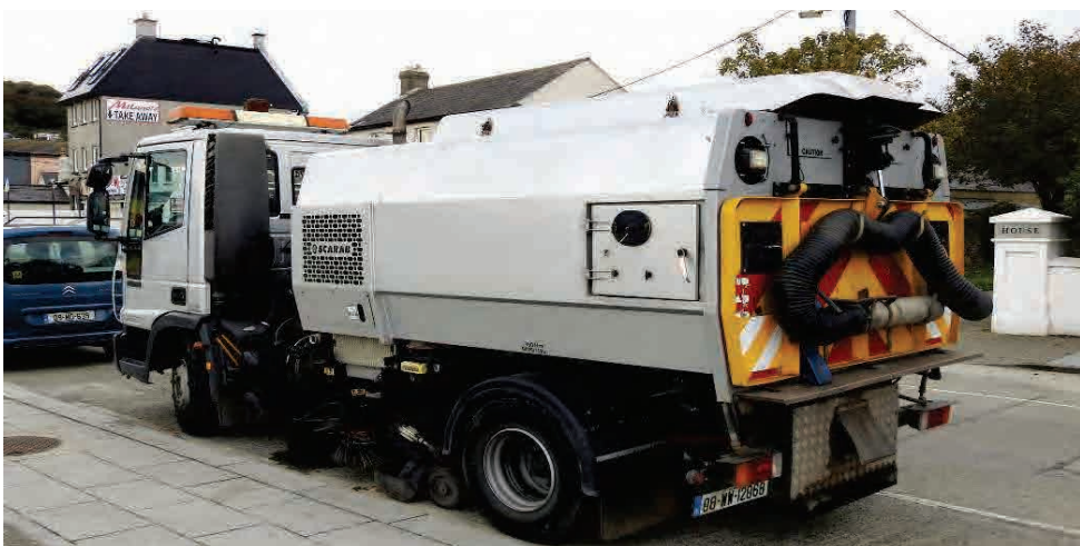
Vacuum trucks specifically made to clean porous pavements
