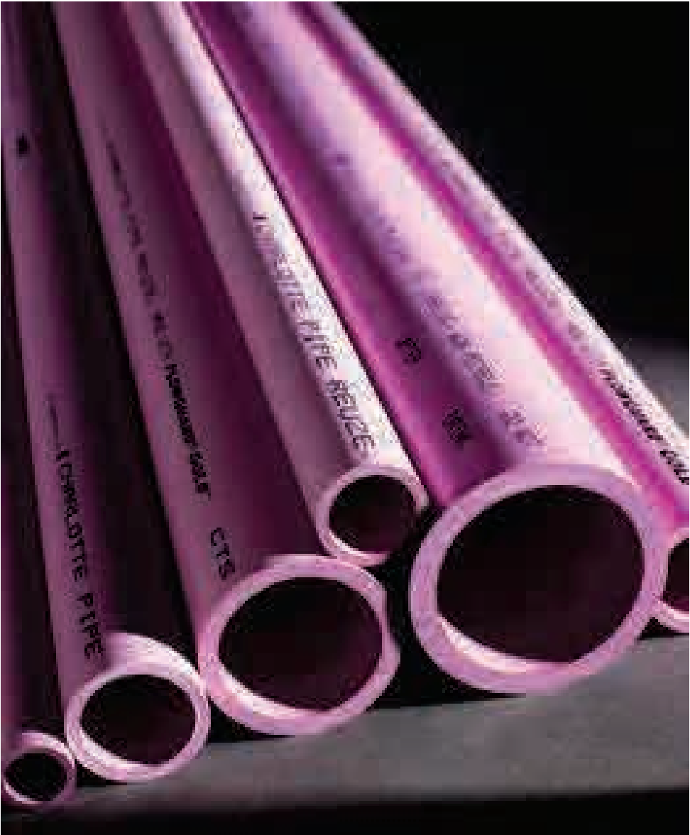
Gray water systems for irrigation use purple pipe to identify them as using non-potable water; the heads, valves, and valve boxes will use the same purple color for identification
