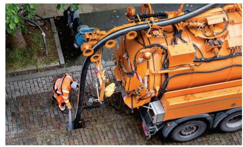
Vacuum truck for cleaning porous pavement
